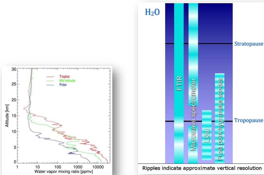
**Figure 2:** Left: Typical water vapor profiles for polar, mid latitude, and tropical regions obtained by frost point hygrometers. Right: Vertical ranges of measurement coverages for frost point hygrometers, lidars, microwave radiometers, and FTIR. Frost point hygrometers and lidars have high vertical resolution, microwave radiometers an intermediate resolution and FTIR only coarse resolution in the troposphere. All instrument types can provide an estimate for the total water vapor column.
